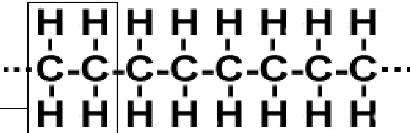
The C=C double bond in an ethylene monomer is transformed into a C-C single bond in the polymer.
