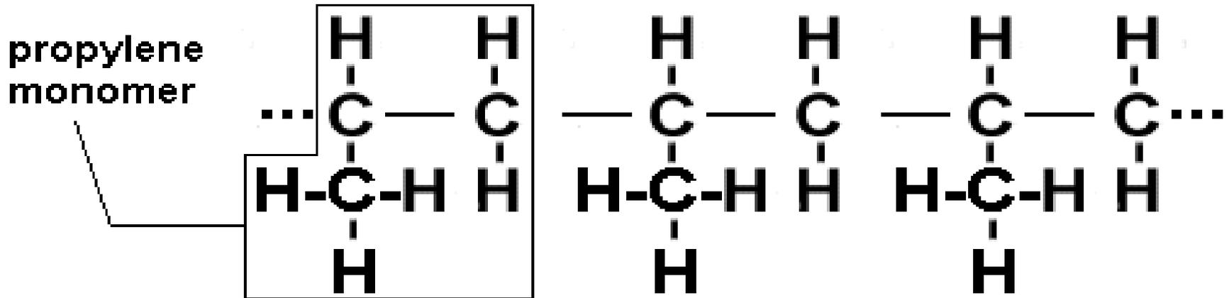
The C=C double bond in each monomer is transformed into a C-C single bond in the polymer.
