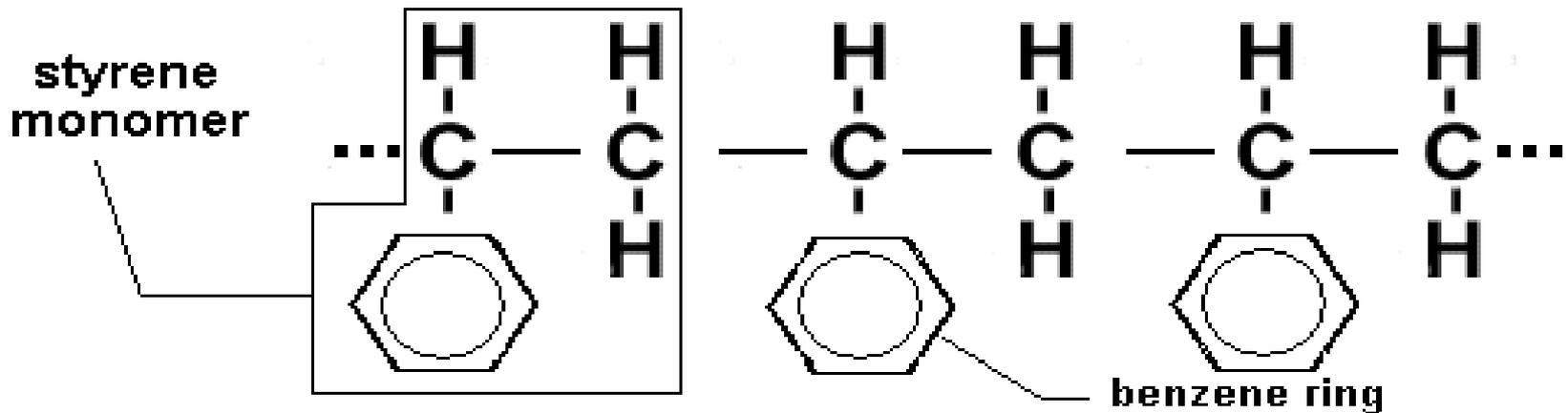
The C=C double bond in each monomer is transformed into a C-C single bond in the polymer.
